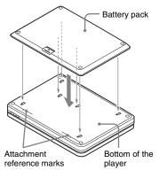
Slide the battery pack in the direction of the arrow until it clicks into place.
